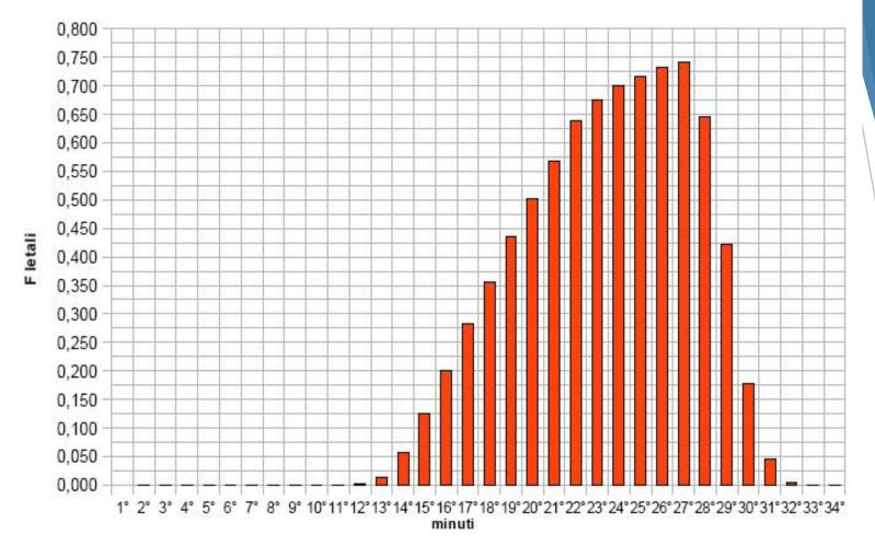
Thermal contribution during a sterilization process.
