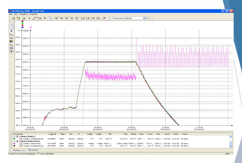
A typical sterilization plateau shows always small fluctuations at 121,1°C.
