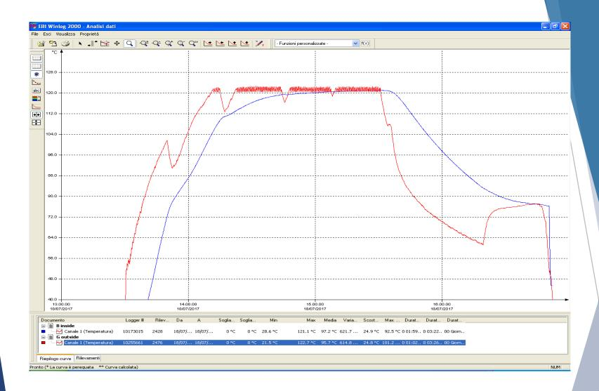
Error in maintain of steam into the chamber, but process ends at the achieving of the F value targeted.
